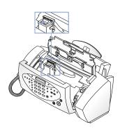
Insert the Cartridge in the Carrier, then push it firmly until it clicks into place. If the Cartridge moves loosely in the Carrier, it has not clicked into place. Repeat this step.
